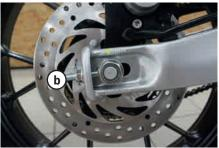
**b)** Loosen the two chain tensioners to create the largest possible chain sag.
