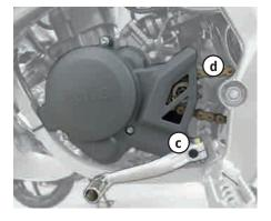
**e)** Now reassemble the cover and the gear lever. When reassembling please make sure to restore the prescribed chain sag of 30 - 35mm. You can easily check this with a folding rule. In addition, you must tighten the rear wheel axle with the intended torque of 78 Nm.
